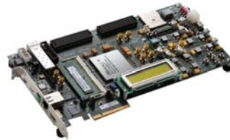
Xilinx Virtex-7 FPGA VC707 Evaluation Kit ( http://www.xilinx.com )
